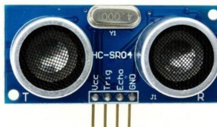
Gambar 34 Sensor ultrasonik
