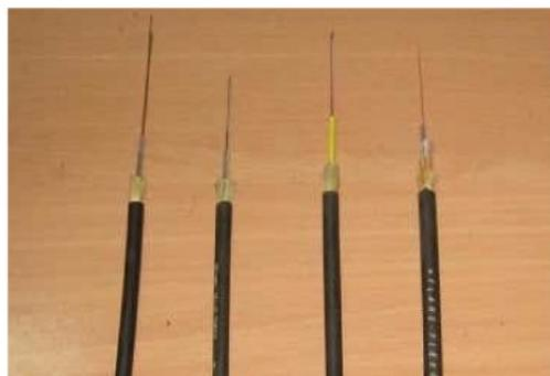
Gambar 2. 26 Kabel Fiber Optik Jenis Patch Cord
